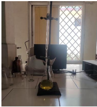
Fig 4 Titrate water with sodium thio sulphate
