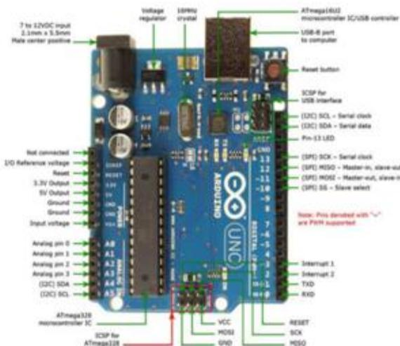
Figure 5: Schematic Pin diagram for Arduino Uno Board
