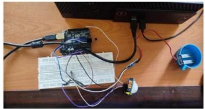
Figure 11: Connection of sensors with Arduino uno
