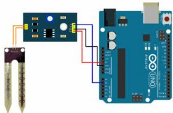
Figure 7: LM393 Soil Moisture sensor with Arduino Uno
