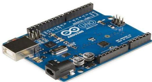
Figure 4: Arduino Uno Board
