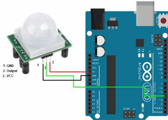
Figure 8: PIR sensor connected with Arduino Uno
