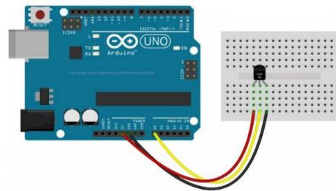
Figure 6: LM35 Temperature sensor with Arduino Uno
