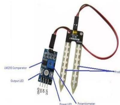
Figure 2: LM393 Soil Moisture Sensor
